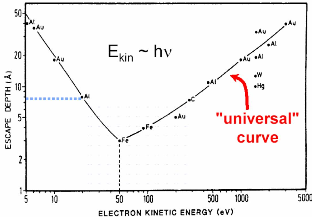
→ ARPES is a **surface technique**: one needs **clean surfaces** + work under **ultra-high vacuum** (better than  $10^{-9}$  Torr).
