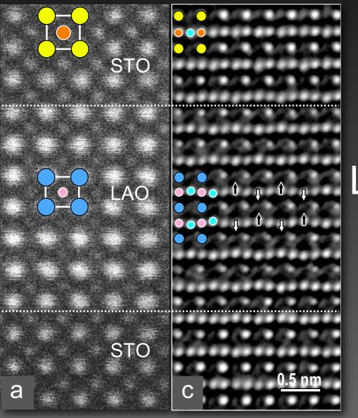
Structural distortion of LAO propagates in several layers of STO at the interface
