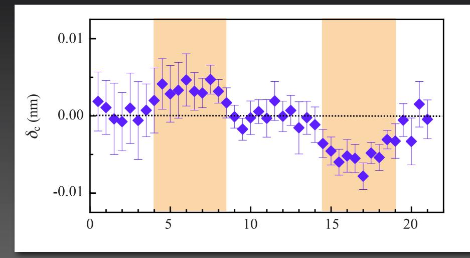
Shift of the center of the oxygen octahedron with respect to the appertaining cations
